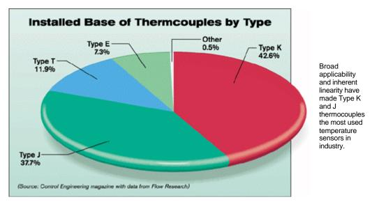
According to the second diagram, types K and J are used in far greater numbers than other junction types, such as T and E. Others include more specialized types like S, R, and B. Greater use of types K and J probably results from their high linearity and ability to provide a high mV over a given temperature range.
